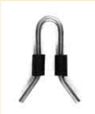
Fig. 7: This is an example of a compressible sleeve used to reduce stone anchor rigidity when the anchors are epoxied in the stone.
