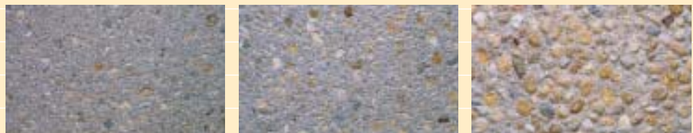
Examples of light, medium and heavy sandblast textures.
