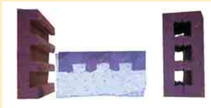
Kerfed brick with a dovetail core allows easy splitting of the brick and a good mechanical bond to the concrete.
