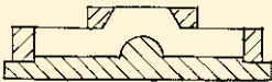
C: INVERTED ARRISE Additional formwork plus additional labor to daily remove and replace back pans.
