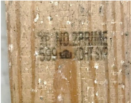
Figure 11 – Grade mark of 2x4 missile
