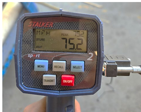
Figure 13 – Radar gun used to record missile speed
